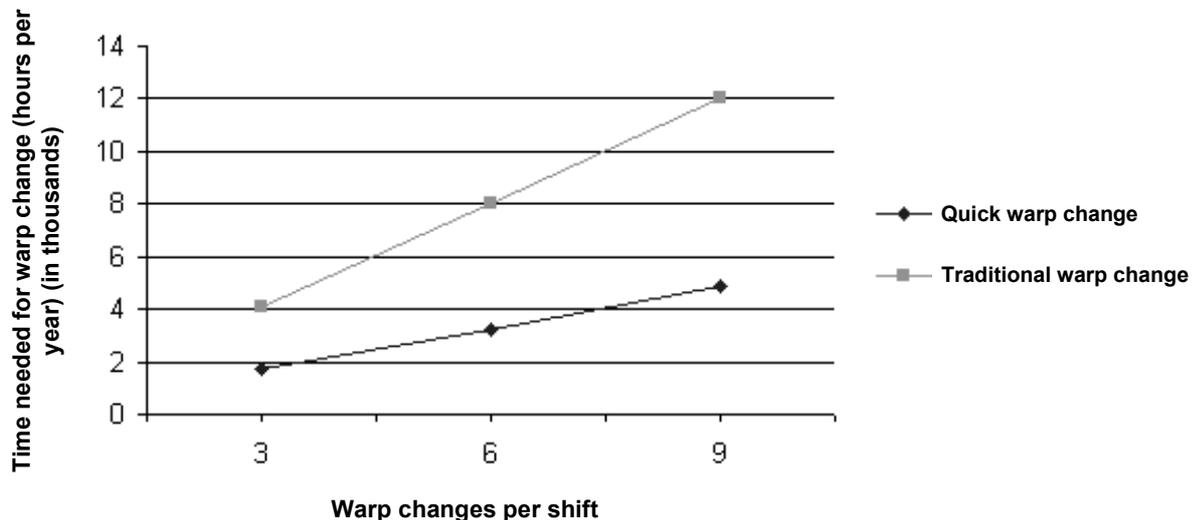
Fig. 95 – Time needed for warp changes during one year in a weaving mill with about 150 machines
