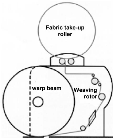
Fig. 103 – Structure of the multiphase multilinear weaving machine
