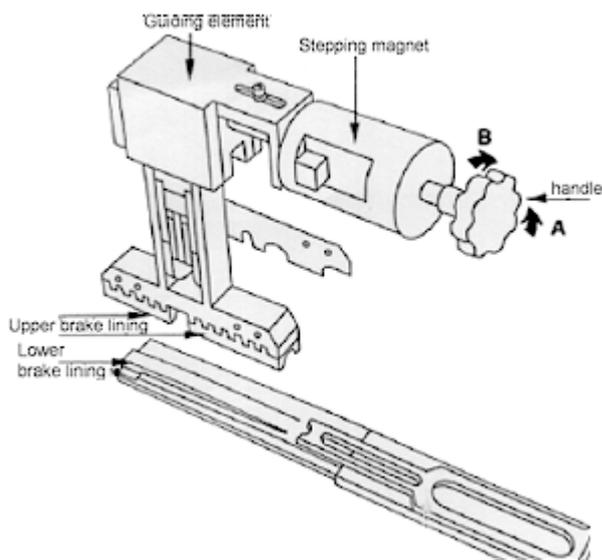
Fig. 51 – Projectile brake
