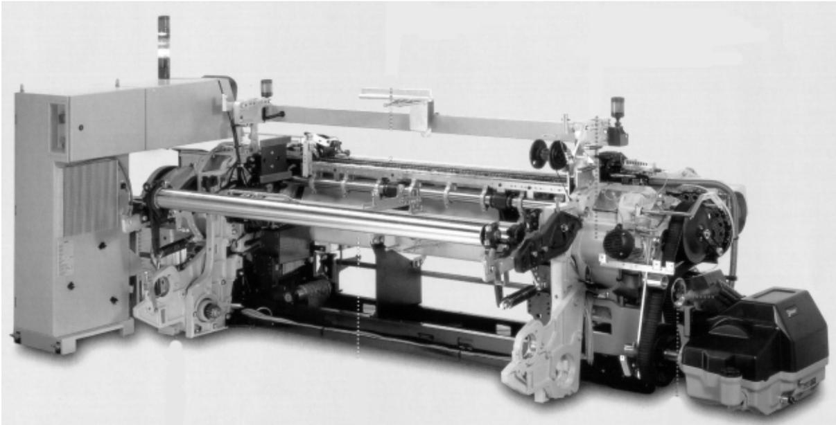
*Fig. 75 – Skeleton of a weaving machine with various already mounted components*
