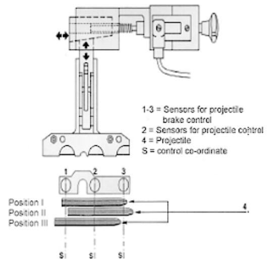
Fig. 52 – Brake adjustment
