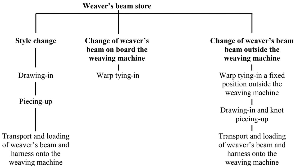
**Changing style** means producing a new fabric style, **weaver's beam changing** means going on weaving the same fabric style just replacing the empty beam with a full beam of same type.
