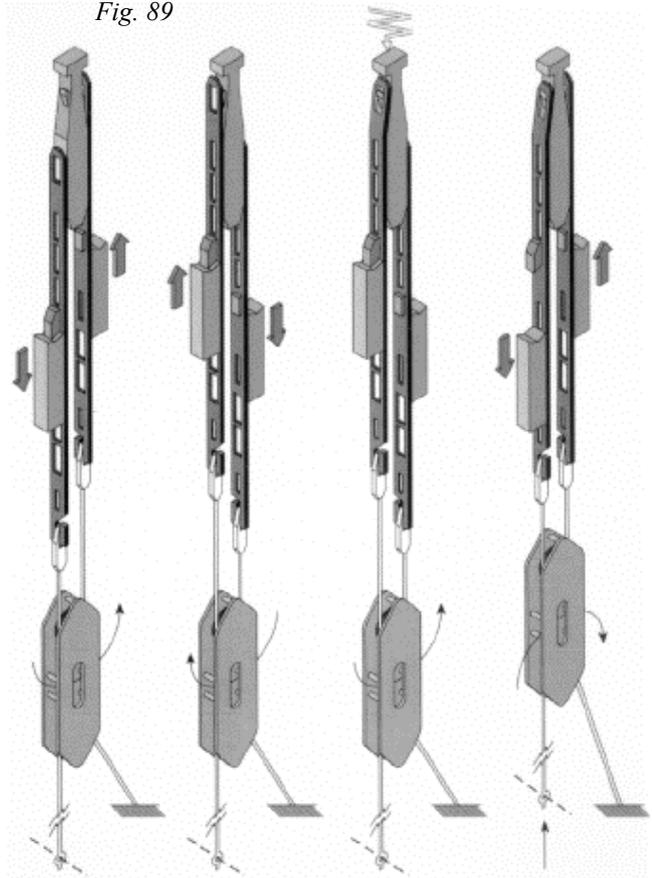
of the hooks). The last two sequences of Fig. 89 show that, when a thread needs to be raised, the magnet receives the impulse and the flexible hook hooks-up to the magnet. This causes the lifting of the double pulley, as in this case it is not possible to make any compensation.
