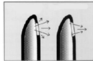
Fig. 57 – Multihole relay nozzles
