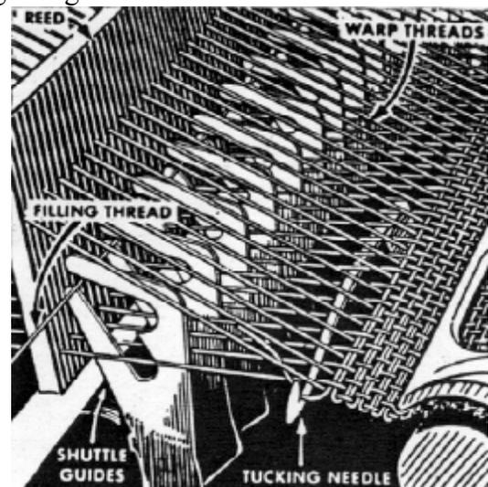
This system is generally used for light to middle weight fabrics, when weave and fabric density permit. There are also available tuck-in selvage motions which are entirely controlled by pneumatic or mixed pneumatic and mechanical devices.
