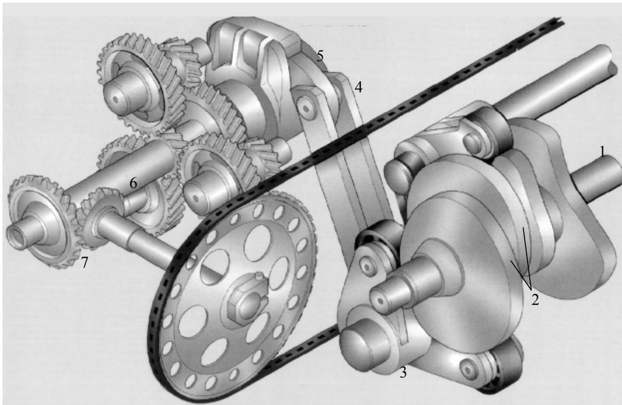
*Fig. 40 – Driving system by double conjugated cams*
