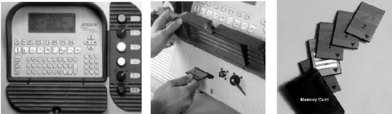
Fig. 91 – Board computer equipped with memory card
