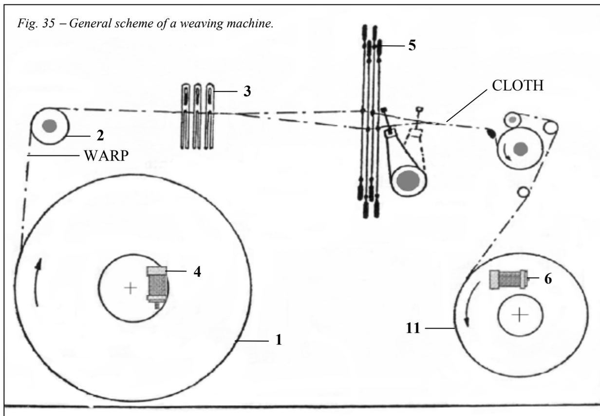
The warp threads wound on a beam (1) are bent on the back rest roller (2), support special drop wires (3), pass through the healds (5) and through the dents of the reed (8) fastened to the slay (7), along which the vehicle transporting the weft runs (9). The fabric produced is then drawn by a take-down roller(10) and wound on the cloth beam (11).
