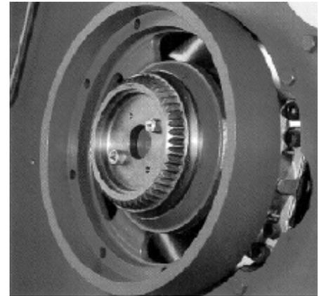
*Fig. 21 Conical toothing.*
