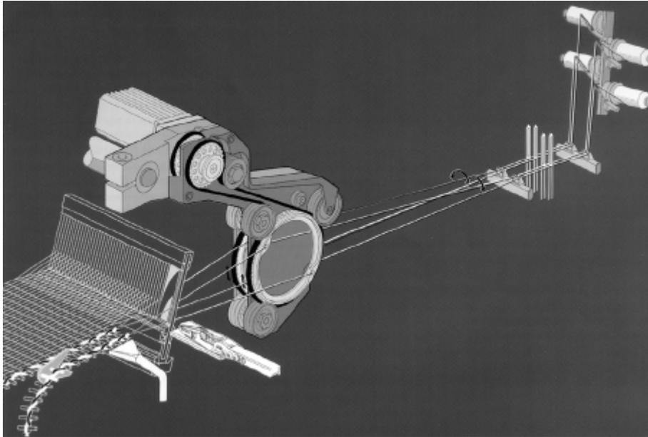
*Fig. 116 – Double disk device for leno selvedges*
