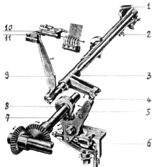
Fig. 48 - Projectile launching mechanism
