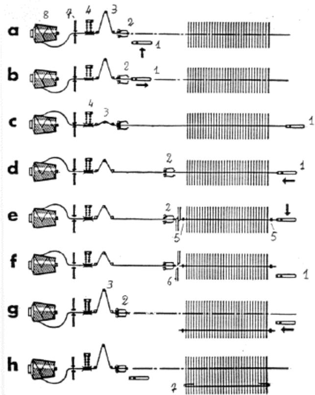
Fig. 50 – Insertion cycle of the projectile machine
