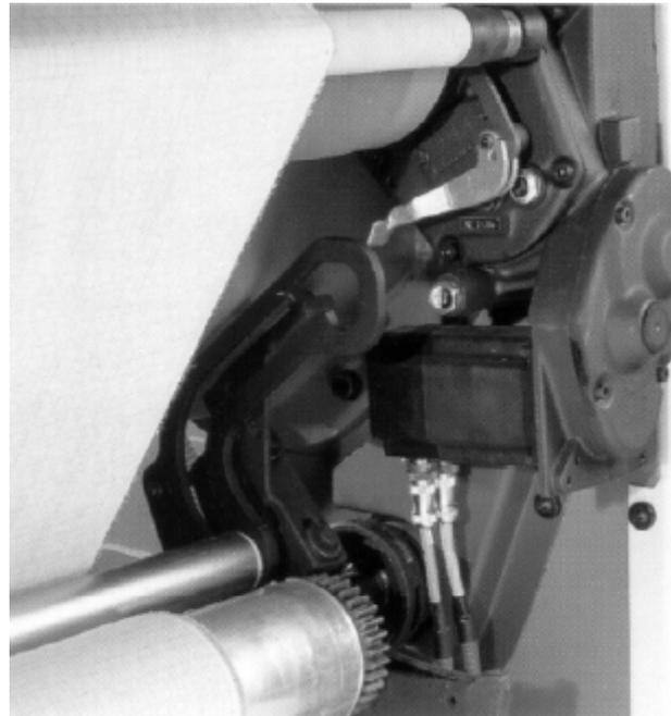
Fig. 78 – Servomotor for take-up motion drive
