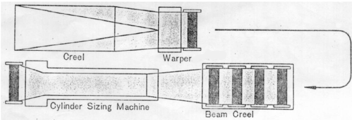
*Fig. 26 – Conventional sizing: Creel: contains the cones
