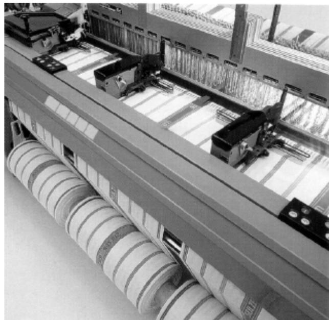
*Fig. 117 – Devices for centre selvedge formation in a projectile weaving machine*
