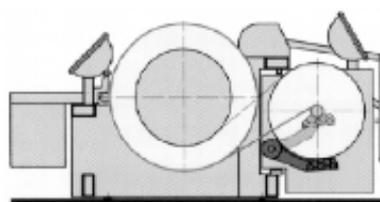
Fig. 16b – Beaming of staple yarns warps with pressure roll device.
