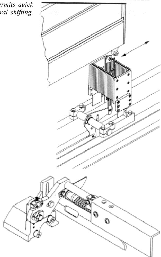
Fig. 99 – **Quick temple positioning:** this operation permits the immediate re-positioning of the temple during re-assembly
