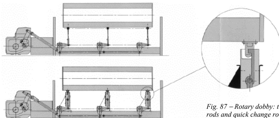
*Fig. 87 – Rotary dobby: traditional rods and quick change rods*
