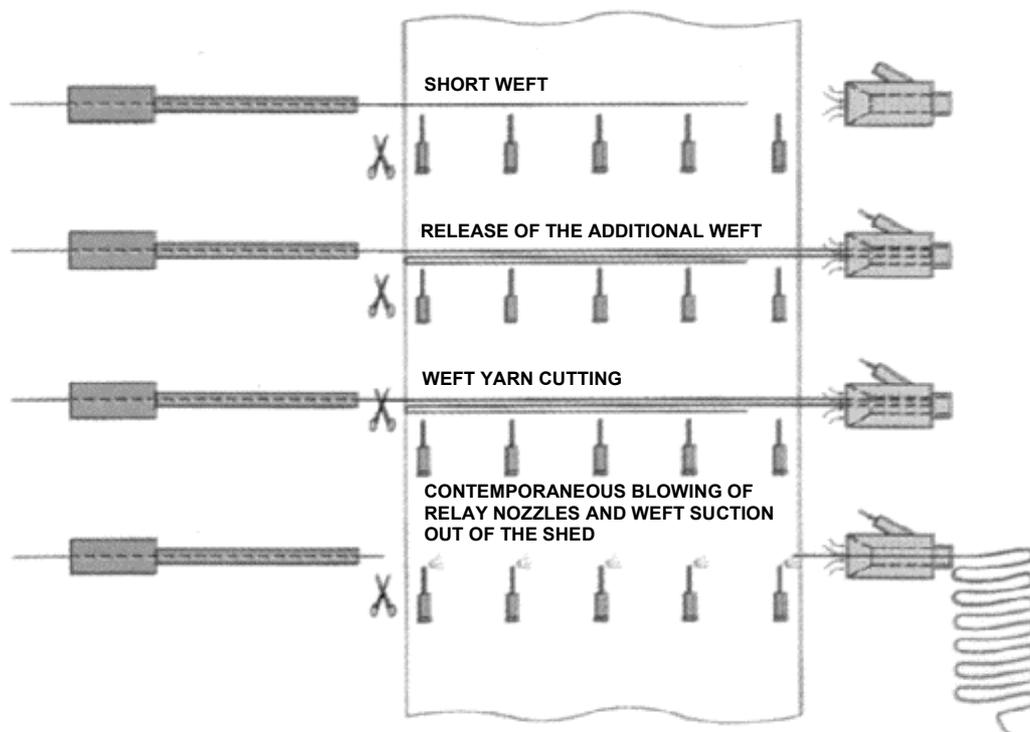
Fig. 59 – Automatic weft repair
