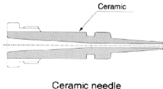
*Fig. 62 – Cross-section of a ceramic nozzle*
