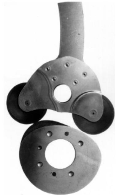
Fig. 82 – Conjugated cams with roller lever
