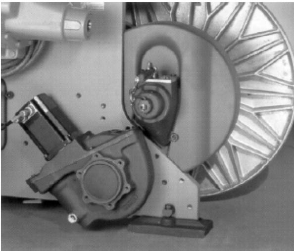
Fig. 77 – Servomotor for let-off motion drive
