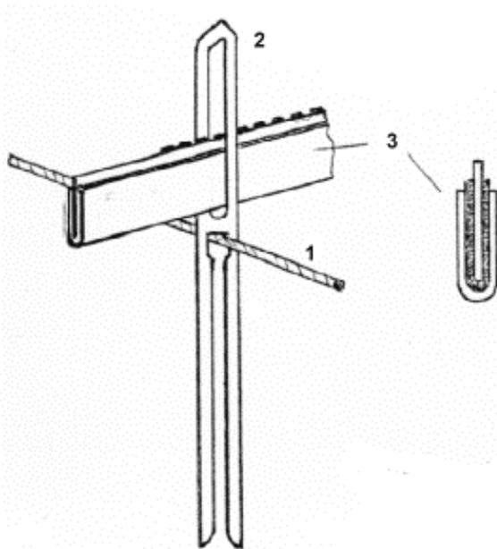
Fig. 110 – Electric warp stop motion:
