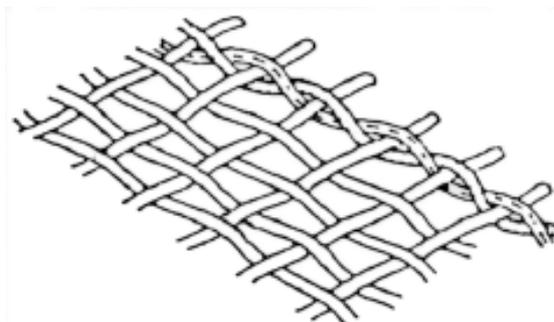
The leno gauze system is optimally suited for heavy fabrics, blankets, wall coverings.
