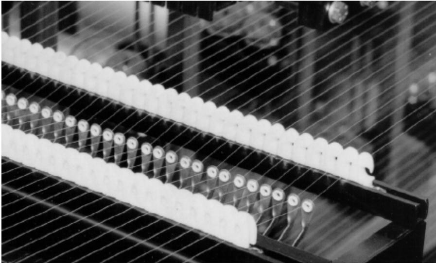
*Fig. 5 – WARP STOP-MOTION WITH OPTICAL SENSING DEVICE.*
