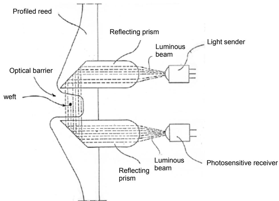
*Fig. 109 – Optical sensor applied on an air jet weaving machine*
