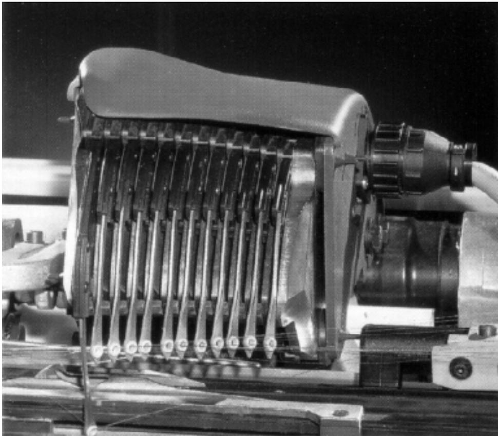
*Fig. 44 – Colour selector with 12 bolts*
