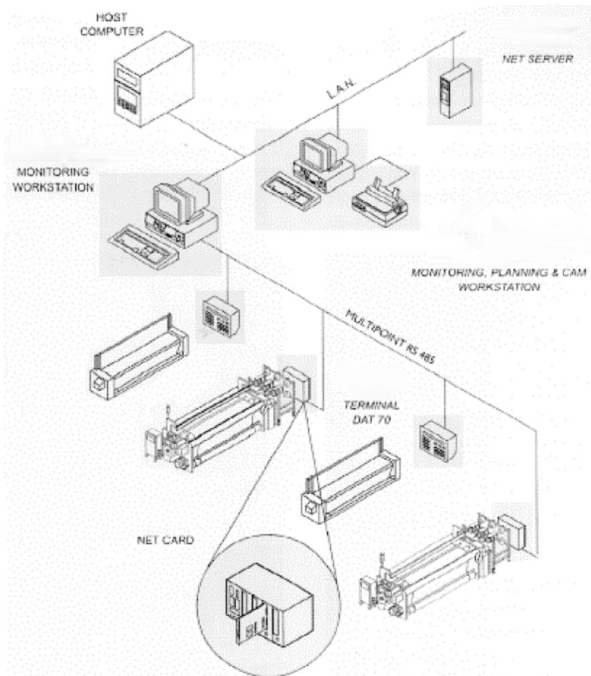
Fig. 118 – Advanced monitoring system
