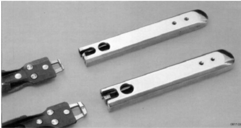
Fig. 45 – **Projectiles:** there are various projectile versions: made of steel, 9 cm long and 40 g heavy, with small section, as suitable for yarns of fine to medium count; made of steel, 9 cm long and 60 g heavy, with large cross-section which, thanks to their higher weight and to the larger clamping section of the gripper, are particularly suited for machines with high reed width or when for weft bulky yarns, as e.g. fancy yarns, are used.
