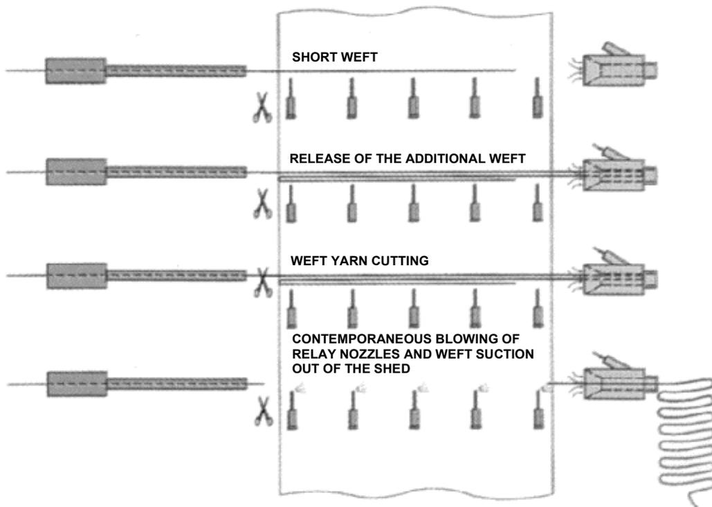
Fig. 59 – Automatic weft repair
