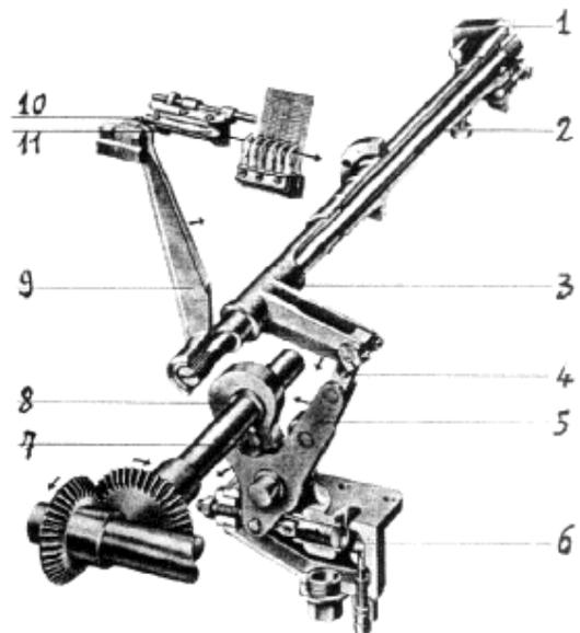
Fig. 48 - Projectile launching mechanism
