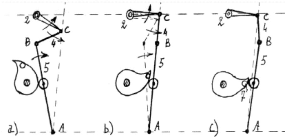
Fig. 49 – Loading of the torsion bar: a) torsion bar 2 in rest, knee-joint lever 4+5 in articulate position; b) loading phase; c) torsion bar in tension and knee-joint lever in stable position, before the launching control by roller 7.
