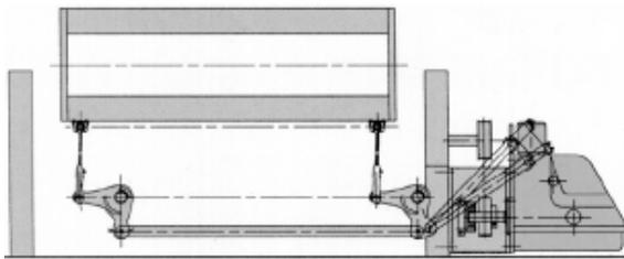
Fig. 81 – Assembly scheme of the cam machine
