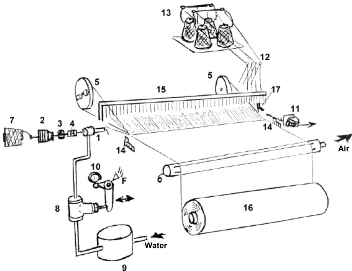
Fig. 60 – Scheme of a water jet weaving machine
