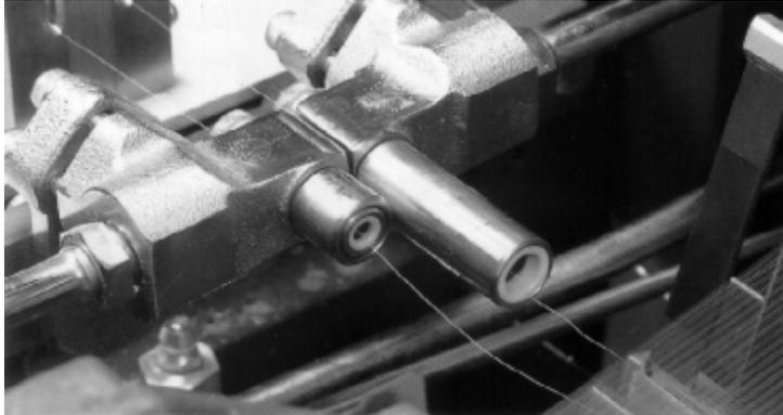
*Fig. 61 – Insertion nozzles for 2 different threads*
